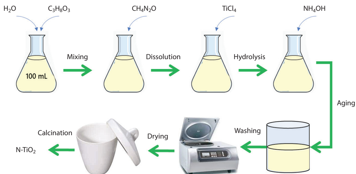
Figure 1 Schematic illustration of the sol-gel synthesis of N-TiO 2 .
