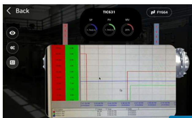
Figure 8 Real-time monitoring of the heat exchanger data
