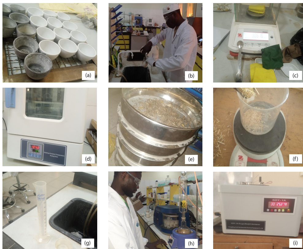
Figure 3 Proximate and energy content analysis: (a, d) weight displacement method for TS, VS, and AC, (b, c, h) lignin, cellulose, and hemicellulose determination for fibre content analysis, (f, g) density, and (i) energy content analysis
