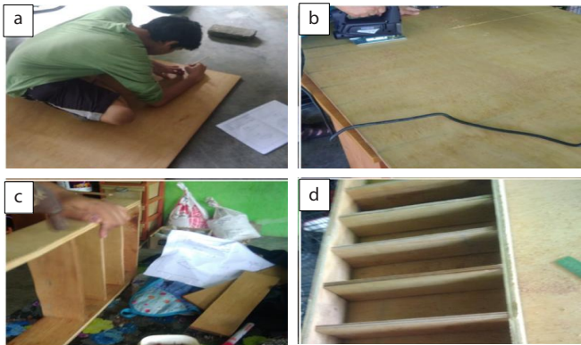
Figure 3 Preparation of brick mould (a) plywood measurement, (b) plywood cutting, (c) nailing the mould, (d) brick mould
