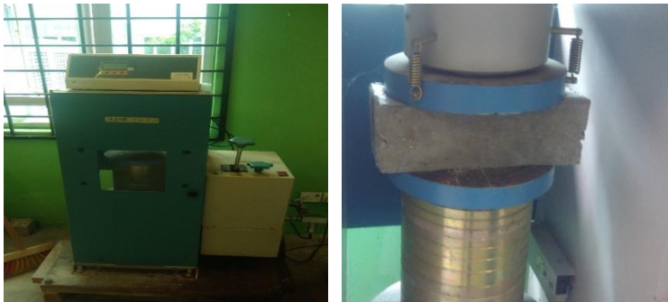
Figure 4 Compression strength machine for brick testing
