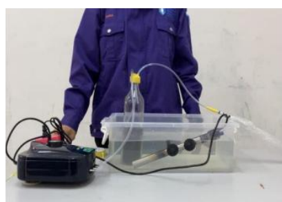
Figure 3 The experimental setup for air stripping pre-treatment
