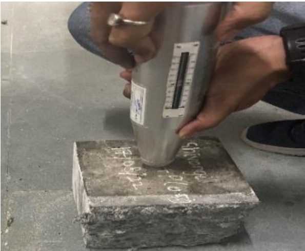
Figure 3 Schmidt rebound hammer test
